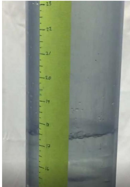
**Figure 5: Water Surface Height at 10 SCFH Air Flow Rate**
