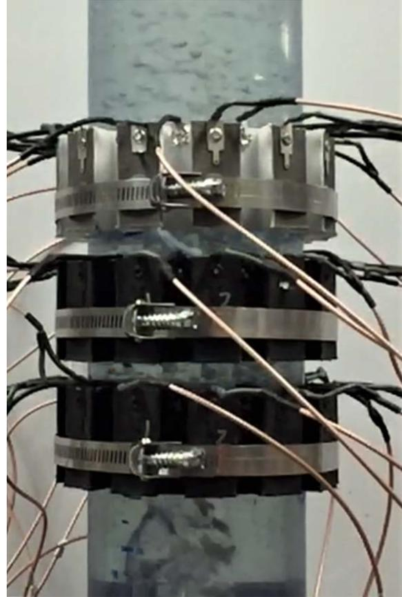
**Figure 3: Sensor on Bubble Column**
