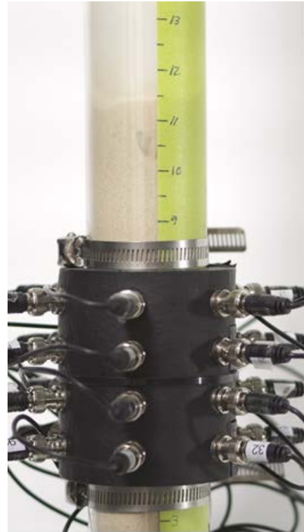
Figure 3: Picture of ECVT sensor around sand fluidized bed column. A rising air bubble can be seen at the 10.5 inch mark.
