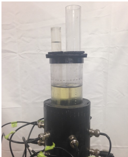
Figure 3: ECVT sensor on oil column with air and water filled inserts
